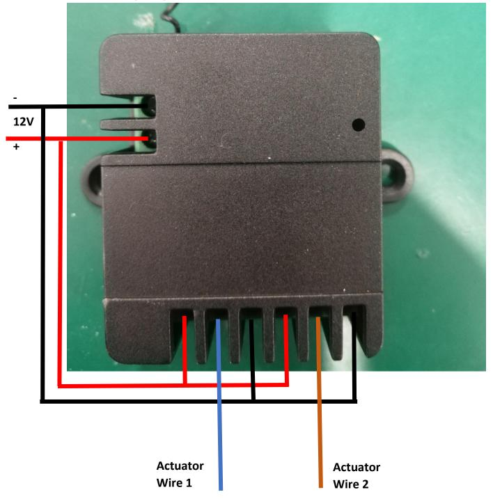
Wire can be connected by the screw terminals or directly soldered on back of PCB, for example
