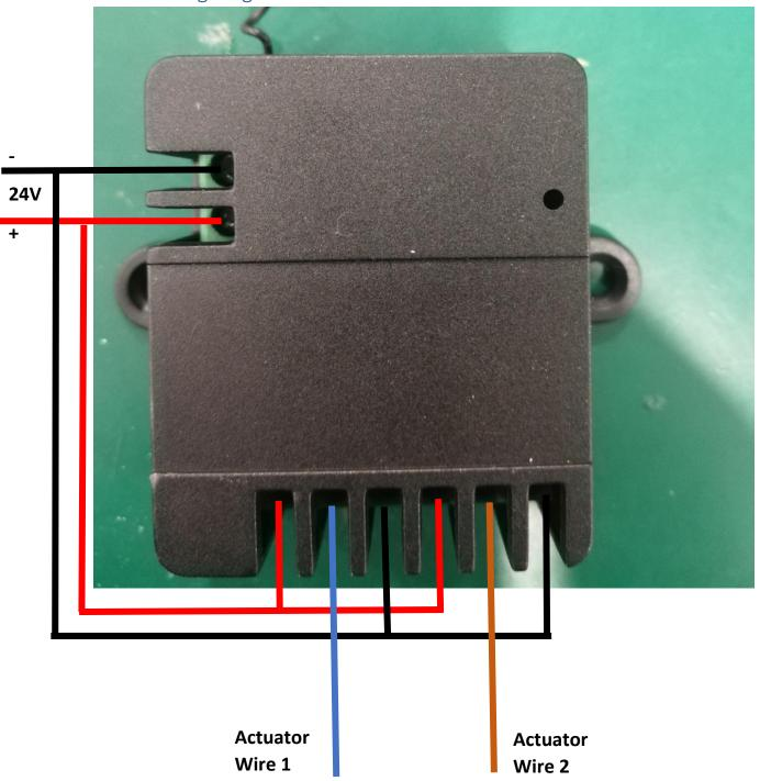
Wire can be connected by the screw terminals or directly soldered on back of PCB, for example
